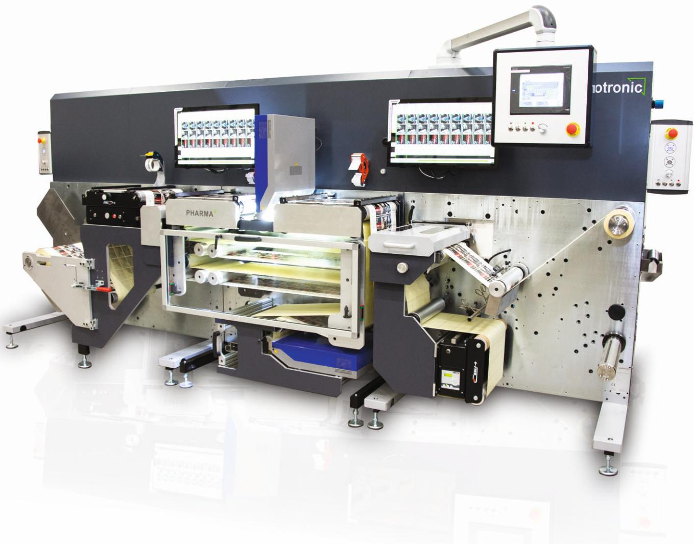
The PHARMA<sup>2</sup> is a new Bi-directional 200% Inspection machine. A servo driven linear buffer reverse the web for fault placement and re-inspection. The buffer movement is ultrafast and precise and guarantees no missed faults detected by the inspection system. Web tension and slitting is unaffected by the reverse movement in re-inspection mode.
